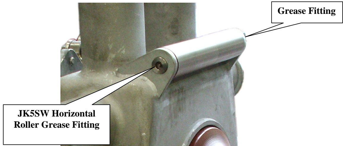
Fig 8. JK5SW Horizontal Roller Grease Fitting Locations
