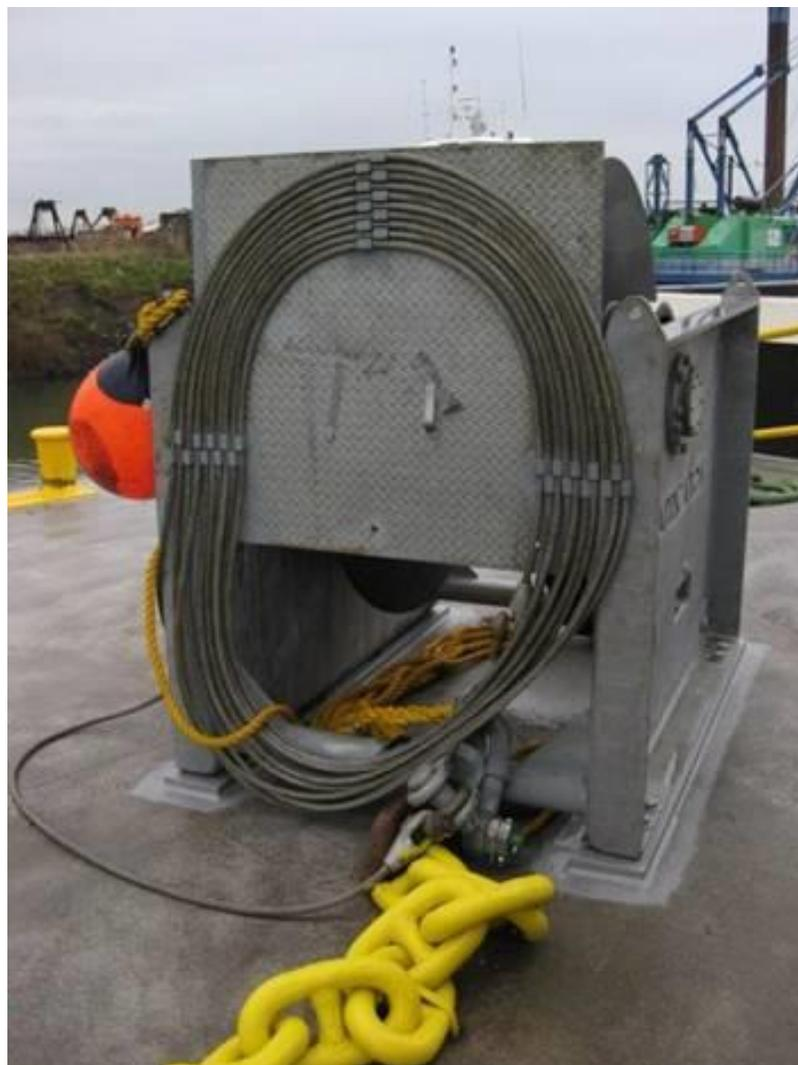
Olympic's order captures several upgrades since the first unit was ordered. A new sprocket-flange allows operators to retrieve deployed cables more easily; thread-down base plates allow for easier mobility for transfer of the unit from barge to barge or to other platforms. Hot-dipped galvanized surface treatment after final assembly finalizes production designed to outlast the barge upon which the unit is installed.
